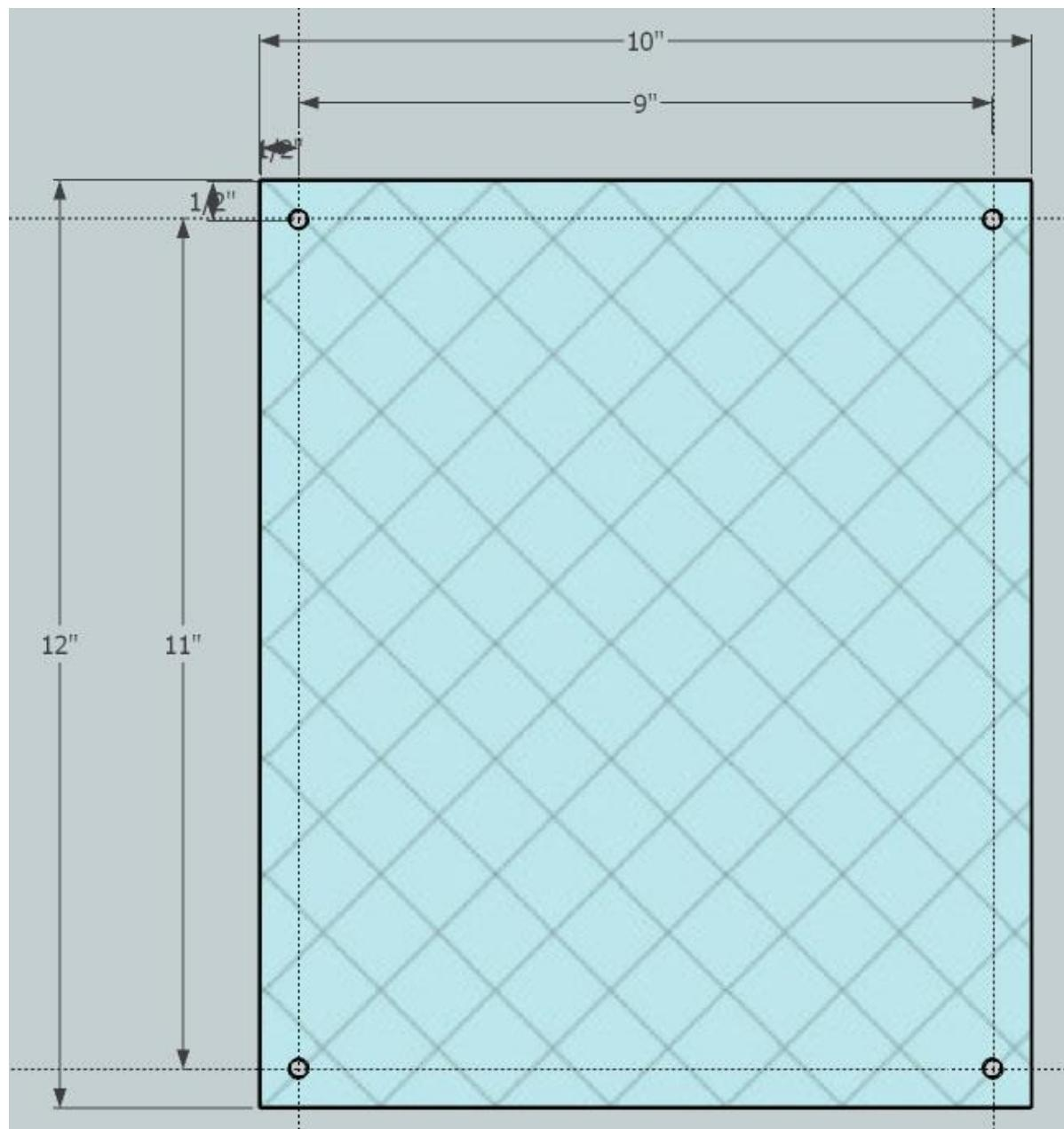
Dry fit the bead board and acrylic together to make sure the holes line up. If the holes are off slightly, drill the holes in the bead board large enough to fit the bolts through.
