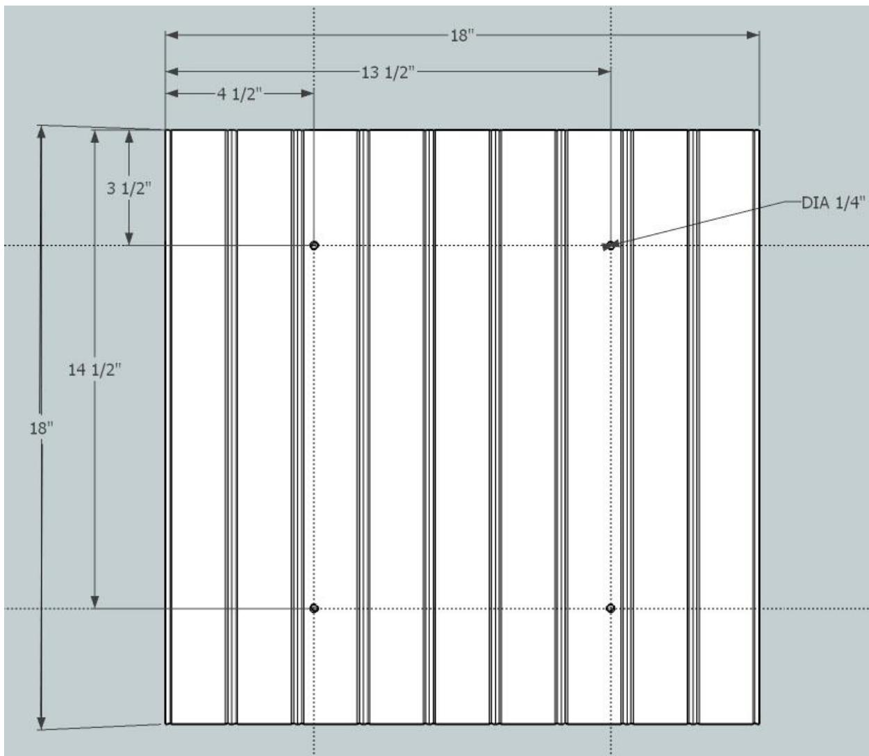
Cut a piece of acrylic sheet to 10" x 12". Note: I use a table saw to cut the acrylic. To minimize chipping, tape the cut zone with painters tape or similar. You can also sand the edges of the acrylic to smooth out small chips. Pick a corner/edge to start all measurements from. Mark the locations for the holes. (See sketch) Drill 4 x  $\frac{1}{4}$ " holes.
