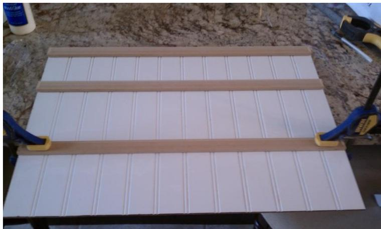
6. Glue the top moulding end caps on. Allow glue to dry minimum 1 hr. Clean off any excess glue.
