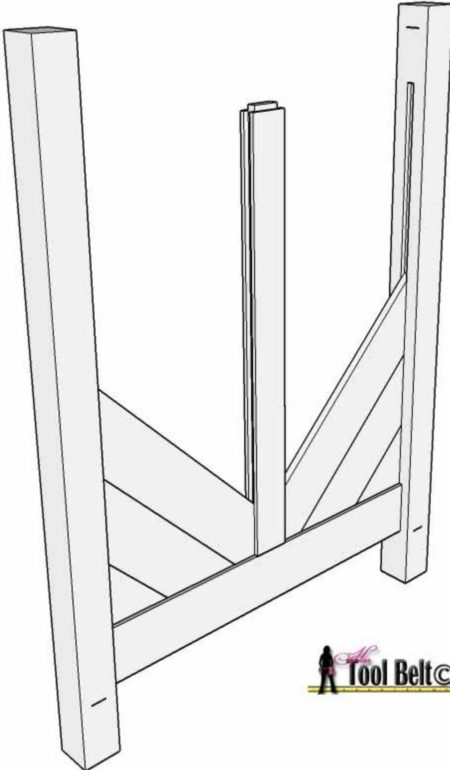
Attach the bed rails to the headboard and foot board 6" up and secure with 2 1/2" pocket screws.
