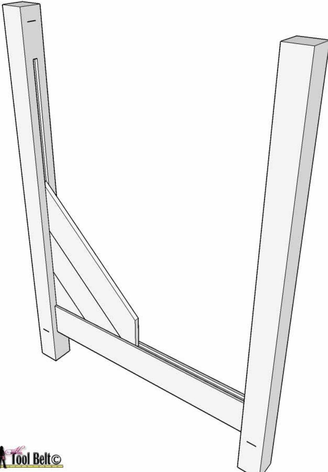
Add the divider and continue to stack the diagonal panels, then top it off with the top rail. Trim any boards as necessary. The diagonal panels will just float in the dado grooves we made. Secure the top rail with 2 1/2" pocket hole screws. Assemble both the foot board and headboard.
