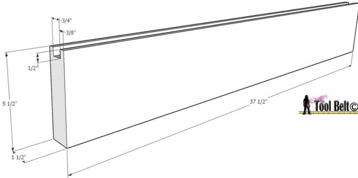
Cut a 2" x 4" x 18" and a 2" x 4" x 42" board. Cut a 3/4" wide x 1/2" deep dado along both long ends. Now we need to cut tongues that will fit into the rail dado's that we just cut. On each end make cuts to match the diagram. The tongue should fit snugly into the rail groove, trim as necessary. These are the head/foot board center dividers. It looks complicated, but it'll make assembly slick and easy.
