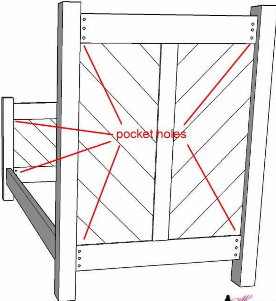
Now let's dryfit everything together and make any adjustments. Attach the bottom rail to the posts 6" up and secure with 2 1/2" pocket hole screws. Stack the chevron panels.
