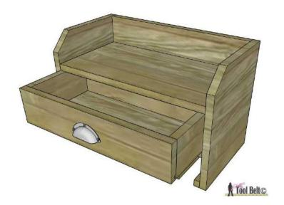
To attach it to the wall, first locate studs in your wall. You'll also probably want it accessible to a power outlet. Once you decide where to hang it, pre-drill holes in the back and attach it to the wall/studs with 3" screws (2 minimum places).
