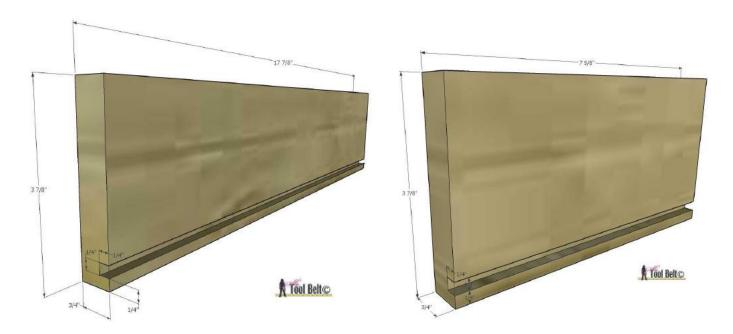
If you have a <u>Kreg Jig® R3</u> (affiliate), you can make pocket joints on each end of the drawer sides (outside) to attach the drawer together. If not, pre-drill holes through the drawer front and back.
