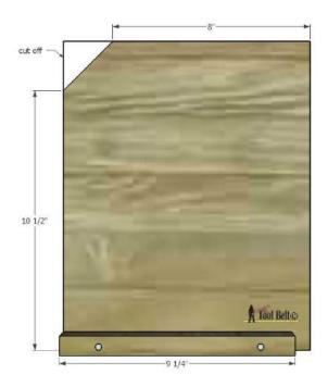
On the sides measure up and mark  $4 \frac{1}{2}$  and  $9 \frac{1}{4}$  from the bottom. The gap between the shelves is 4". Pre-drill the sides, glue and screw the shelves between the sides.
