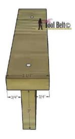
Take one of the shelves. Mark and pre-drill holes to attach the dividers to the shelf. Glue and attach the dividers to the shelf with  $1 \frac{1}{4}$ , make sure the screws are flush or lower with the wood surface. The gap between each divider is 3".
