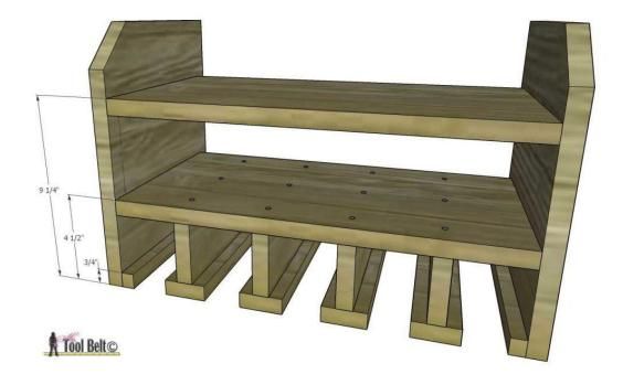
Attach the back, between the sides. Secure with glue and screws.
