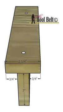
Take one of the shelves. Mark and pre-drill holes to attach the dividers to the shelf. Glue and attach the dividers to the shelf with  $1\,1/4$ ", make sure the screws are flush or lower with the wood surface. The gap between each divider is 3".
