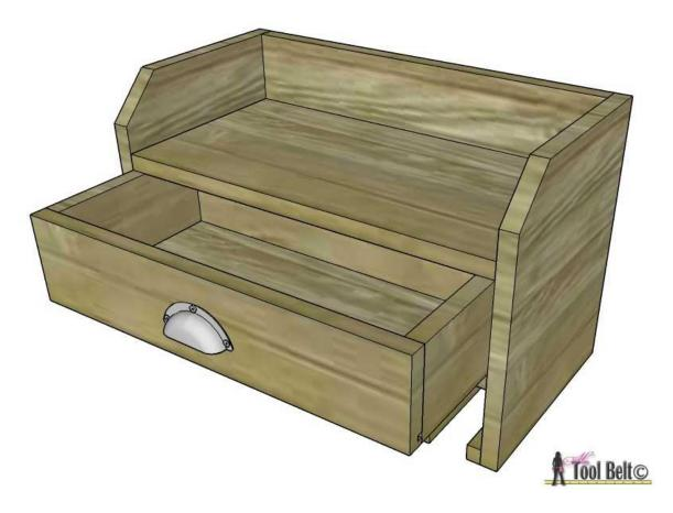
To attach it to the wall, first locate studs in your wall. You'll also probably want it accessible to a power outlet. Once you decide where to hang it, pre-drill holes in the back and attach it to the wall/studs with 3" screws (2 minimum places).
