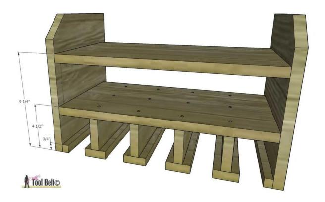
Attach the back, between the sides. Secure with glue and screws.
