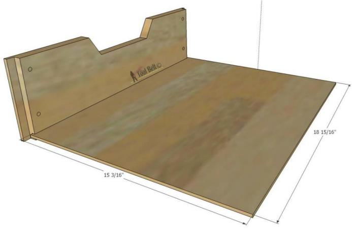
Apply wood glue to the side dados on the front piece and the sides of the back piece. Place the bottom in the bottom dados, place the sides on and secure with 1" or 3/4" pocket hole screws.
