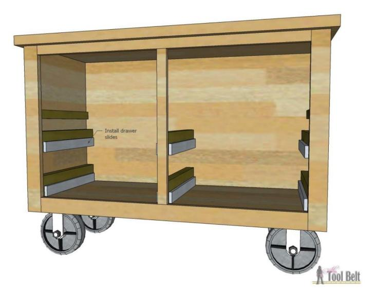
Install the other side of the drawer slides on the drawers and install them into the cabinet, make any adjustments/shim as necessary.
