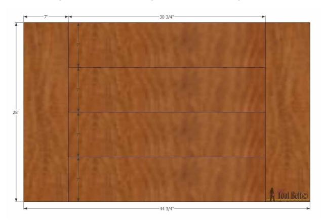
Cut the top pieces, 4 @ 30 3/4" and 2 @ 28". When using 2 x 8 for tops, I like to trim down the sides with a table saw to get a straight edge. The widths of the 2x8's are trimmed down to 7" wide.
