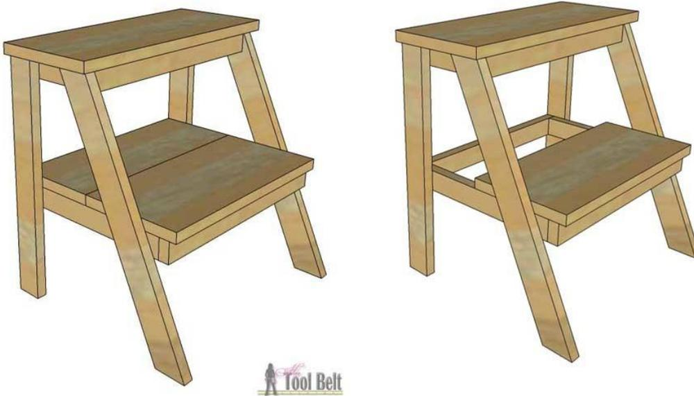
Secure the stair treads to the stool frame with either pocket screws or nail from the top into the frame. The top stair tread is flush on the back and hangs over 1/2" on the sides and front. The lower stair tread is flush on the back and sides and hangs over 1/2" in the front.
