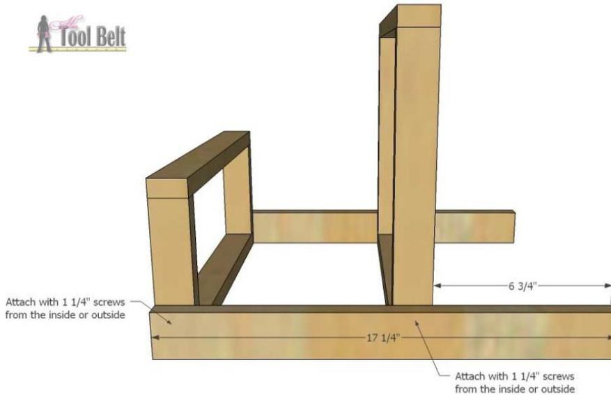
Line up the 19" diagonal pieces with the outside corner of the top stair support, use a screw to secure. Place the stool on a flat surface, mark on the 19" diagonal pieces 6 3/4" from the bottom. Adjust the bottom stair support until it lines up with the marks, clamp into place then secure with screws. Add additional screws to the top support as needed.
