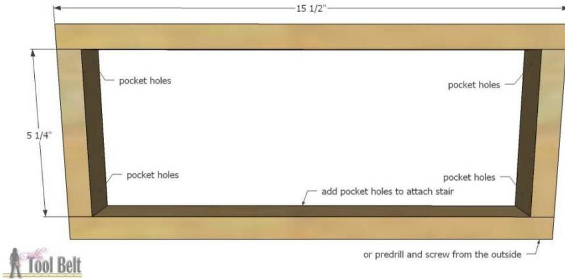
Drill pocket holes in both ends of the 11 1/4" pieces. Use wood glue and 1 1/4" screws to assemble the lower stair support. Add pocket holes to attach the stair tread later.
