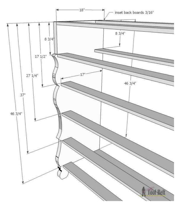
Use wood glue and 1 1/4" pocket hole screws to secure the rails on a side. Make the pocket holes face up on the top 1x4's, and down on all of the other 1x4's.
