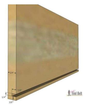
Set aside all of the 3/4" drawer pieces that are 16" long, these are the drawer sides. In all of the other 3/4" pieces, drill pocket holes for 3/4" material in the opposite face of the dado, avoid putting pocket holes by the dado.
