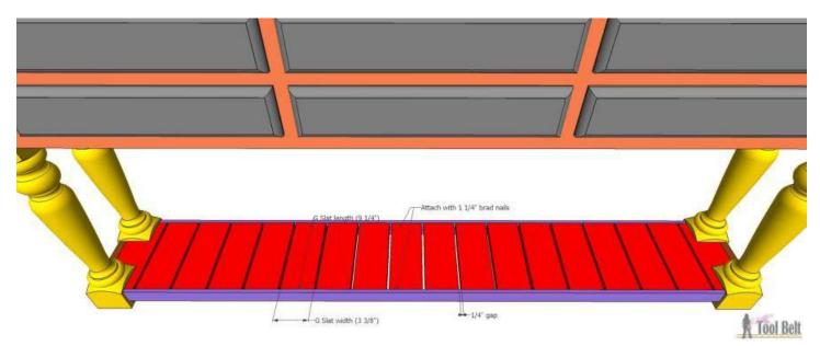
Mark the bottom piece to notch for the legs. A jig saw is an easy way to make the notches. Secure the bottom piece with 3/4"-1 1/4" brad nails.
