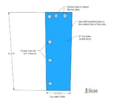
On the legs mark in 1/4" from one side (top and bottom blocks). Mark 29" from the leg top for the bottom side piece to attach. Use wood glue and 1 1/4" pocket hole screws to attach the top side and bottom side to a leg.
