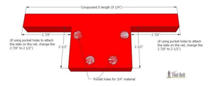
Use wood glue and 1 1/4" pocket hole screws to attach a bottom side to and end slat.
