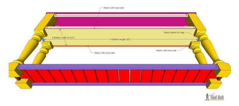
Before attaching the back, you'll want to install the knobs/pulls (this may be after painting/finish). Attach the back with 3/4"-1 1/4" brad nails.
