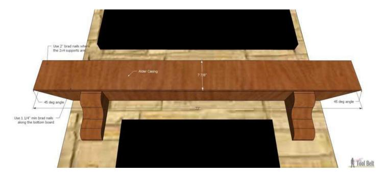
Cut a 45 deg angle on each end of the top board to fit snug against the wall. Use 1 1/4" brad nails to attach the top to the 2x4 supports and to the front board.
