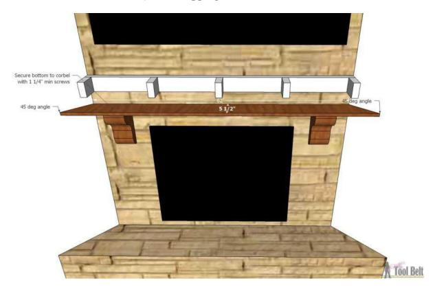
Cut the front board (casing) to fit snug along the bottom board and with a 45 against the walls. Nail the front to the bottom near the bottom edge with 1 1/4" brad nails. Limit the number of nail holes, since they'll show (probably about 4-5). Nail the front to the mantel support 4" 2x4's near the top 2" or so. The crown will cover these holes.
