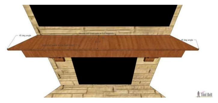
Cut the crown molding to fit under the top. Nail the crown in place, with as minimum nails as possible.
