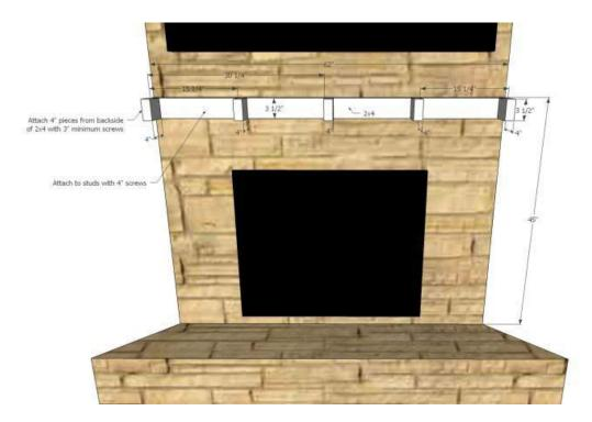
Cut a piece of 2x4 to 62" and cut 5 pieces that are 5" long. Spread the 4" pieces evenly along the 2x4, and secure from the back of the 2x4 with 3" screws (make sure they are countersunk or sucked into the wood). Mark the studs in the fireplace wall, level and attach the mantel support into the studs with 4" screws. (I attached it at 45" from the step)
