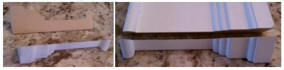
c. In the 24" top molding cut 2 rabbet joints. On the backside at the bottom, cut a rabbet that is  $\frac{1}{16}$ " deep and 1  $\frac{1}{16}$ " high. (I usually cut these with multiple passes on the table saw.
