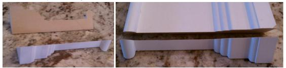
c. In the 24" top molding cut 2 rabbet joints. On the backside at the bottom, cut a rabbet that is  $\frac{1}{16}$ " deep and  $\frac{1}{16}$ " high. (I usually cut these with multiple passes on the table saw.
