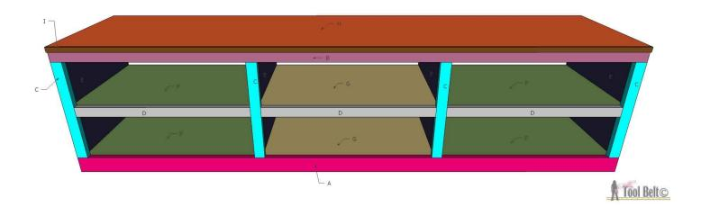
Cut pieces A, B, C and D for the face frame. Drill pocket holes in both ends of the C and D pieces, as shown. Reference K and L measurements from the spreadsheet. Use wood glue and 1 1/4" pocket hole screws to assemble your face frame together. Allow the glue to dry, remove excess glue. Add 3 or so pocket holes along the top of B to attach the top later.
