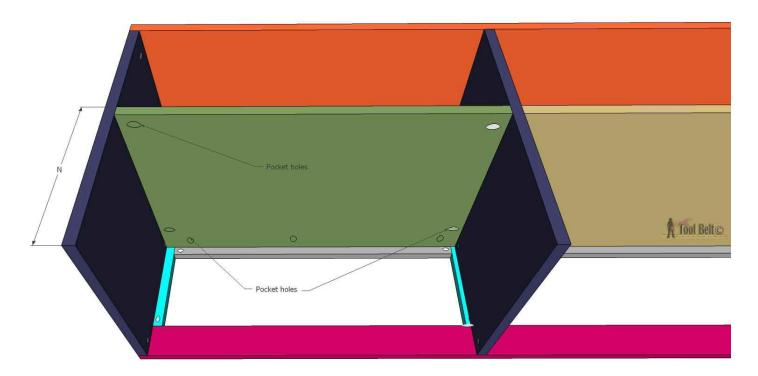
After installing the upper shelves, install the lower shelves. Make the shelf flush with the face frame opening.
