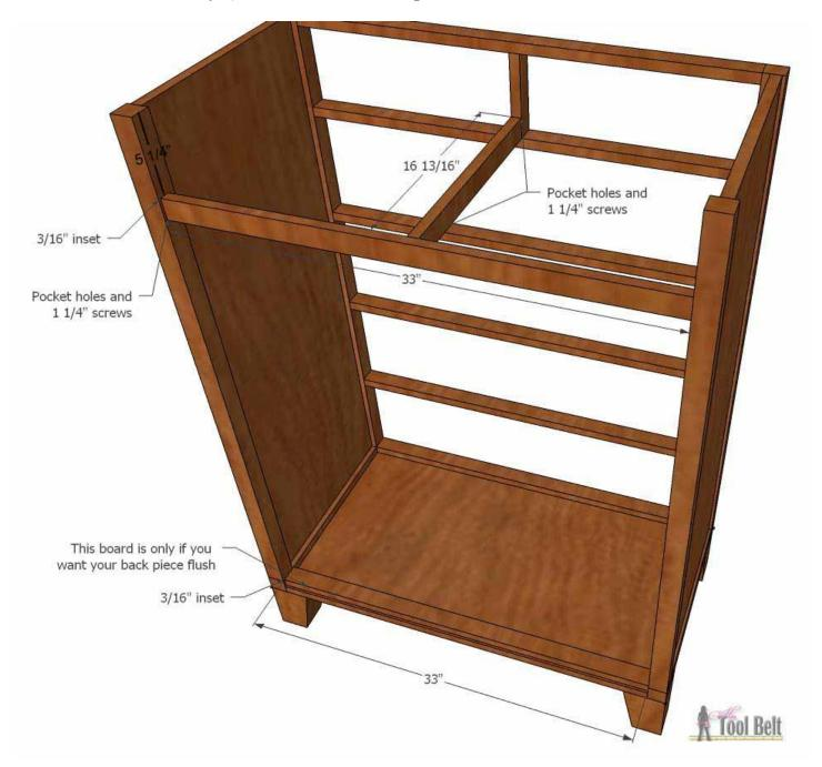
Time to install drawer slides, according to the manufacturers directions. The slides need to start 3/4" from the front face of the dresser. You'll need to take some scrap wood and make 1/2" shims/spacers to make up for the 1/2" inset on the side.
