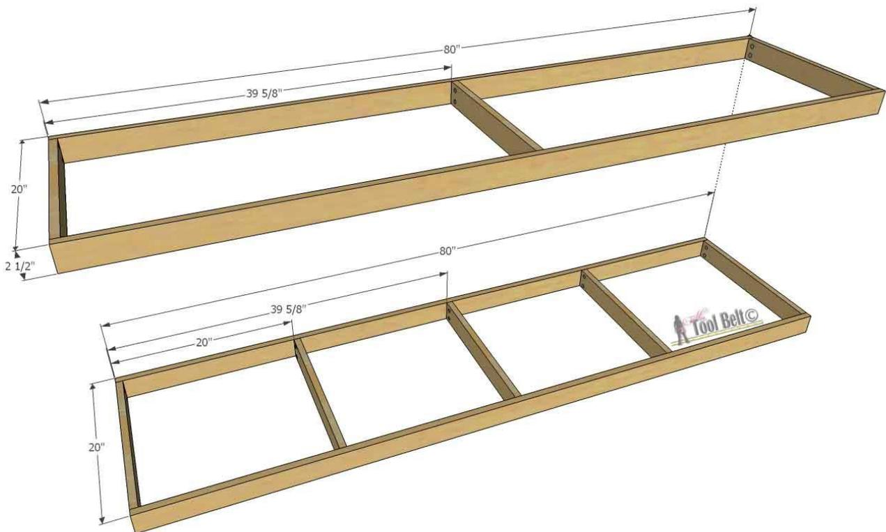
Cut the 1x4s to 80" long. I like to trim the edges until the width is 3 1/4" so I have straight edges to work with. I decided to give the bottom a planked look and left a 1/16" gap between the boards. Use wood glue and 1 1/4" or longer brad nails to secure the boards.
