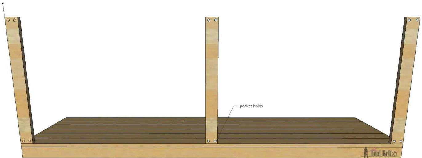
Tip the table onto it's back and clamp a scroll leg into place (flush with an edge). Use 2 or 3 - 2 1/2" screws to attach the leg to the bottom.
