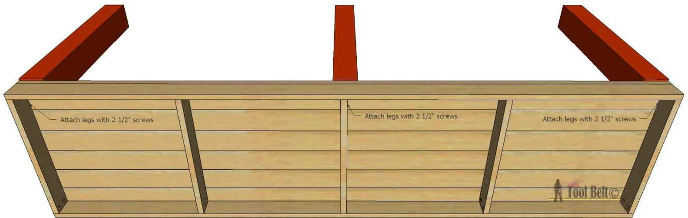
Add pocket holes to the top frame that will attach the top later, and pocket holes to attach the top frame to the scroll legs. Use wood glue and 1 1/4" screws to attach the top frame to the back and legs.
