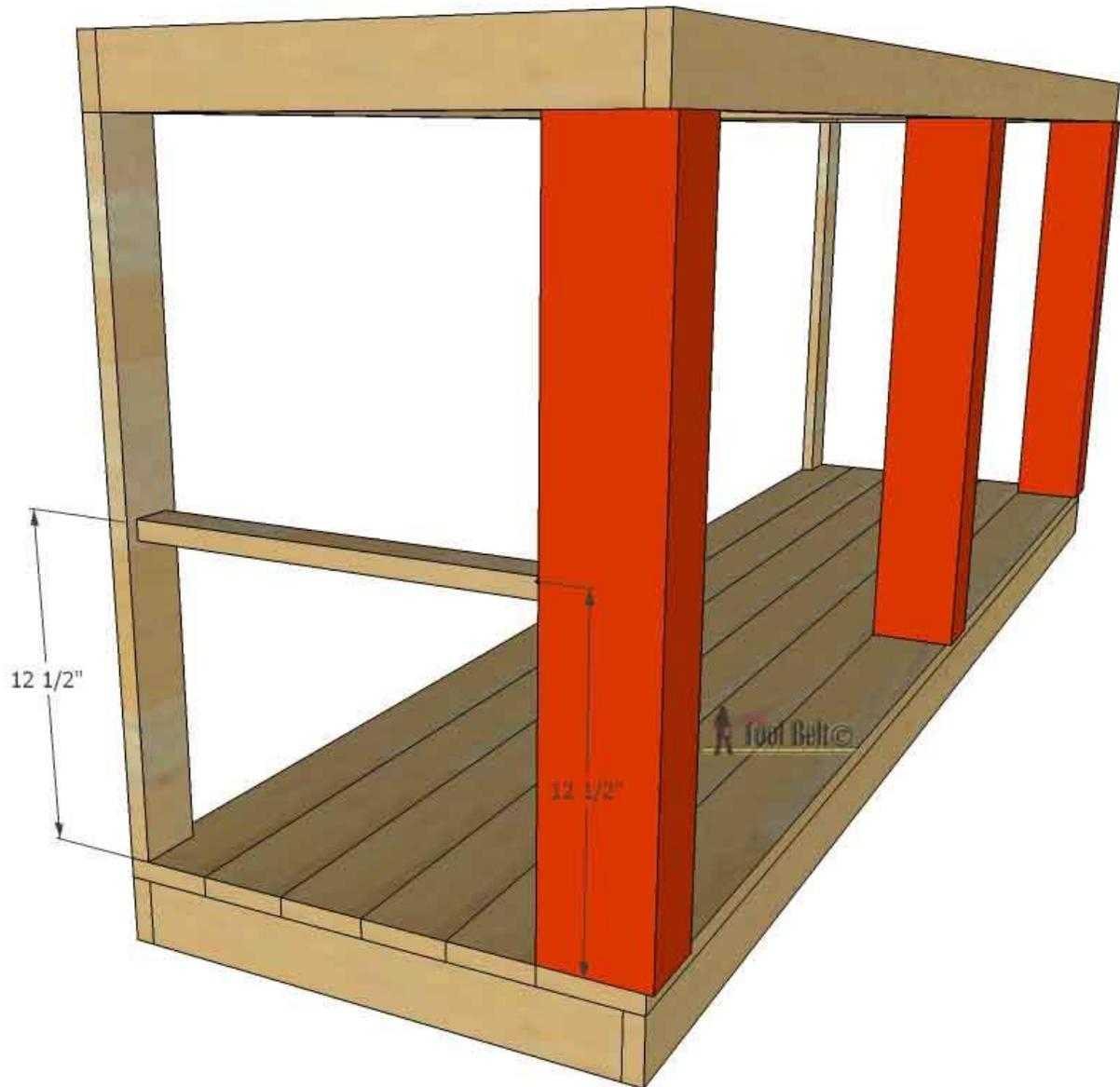
Measure across the length, mine was about 15 5/8" - 15 3/4". Cut a 3/4" x 1 1/4" x your number board with a 20 deg miter. Drill pocket holes on the 90 deg side underneath. Use glue and 1 1/4" to attach it to the back, use 1 1/4" brad nails to attach the other side to the scroll leg.
