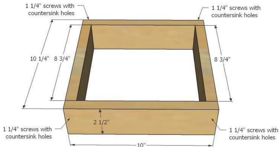
Pre-drill 3 holes in the top 2 1/2" of the chair legs. Use wood glue and 1 1/4" screws to attach the legs to the chair skirt as shown. Tip for getting the chair to not rock. Attach 3 legs to the skirt. Place the
