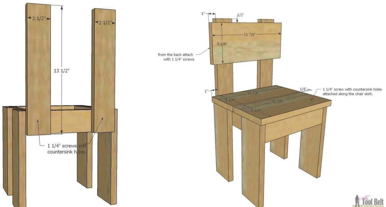
Pre-drill holes in the seats to attach to the chair skirt. Center the seats on the chair frame and secure the seats with 1 1/4" screws. Offset the back from the top of the back support about 1/2" and secure with 1 1/4" screws.
