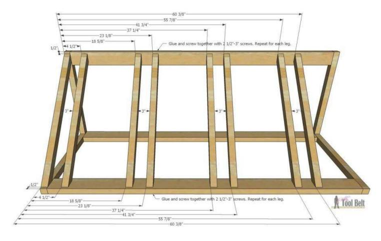
Measure and mark the location of the scooter supports on the base. Pre-drill holes for the scooter supports and secure with wood glue and 2 1/2" screws.
