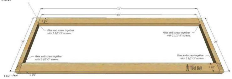
Attach a 24 1/2" board to each end of the remaining 69" board, secure with wood glue and 2 1/2" screws to create the back.
