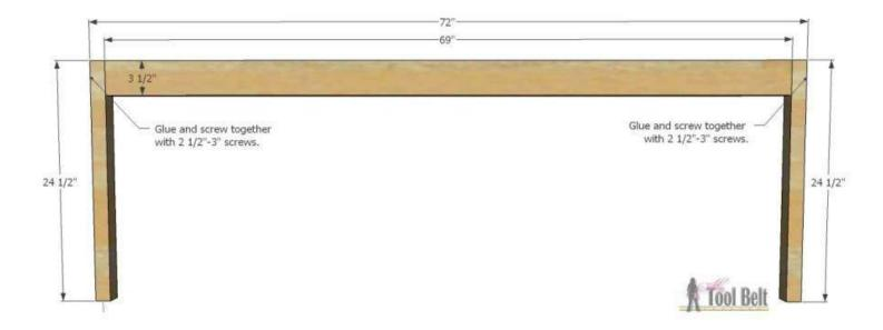
Attach the back to the base, secure with wood glue and 2 1/2" screws. Keep the back flush with the back of the base.
