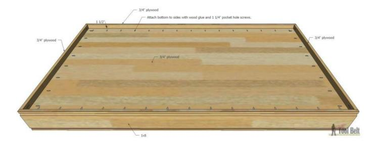
Use wood glue and  $1\,1/4$ " pocket hole screws to secure the side pieces to the front and back.
