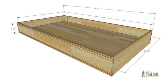
If you are building the trundle for an existing bed, adjust the length to fit under the bed.
