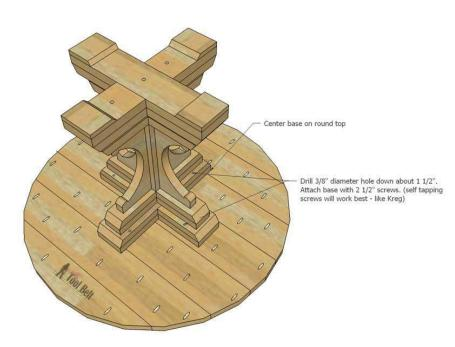
**Step 13 -** Place the pedestal base upside down on the table top and center the base. In the 24" 2x6 base pieces, use a 3/8" drill bit (the pocket hole drill bit) and drill down about 1 1/2" in a few places. Use 2 1/2" self tapping screws (Kreg) to attach the pedestal base to the table top.
