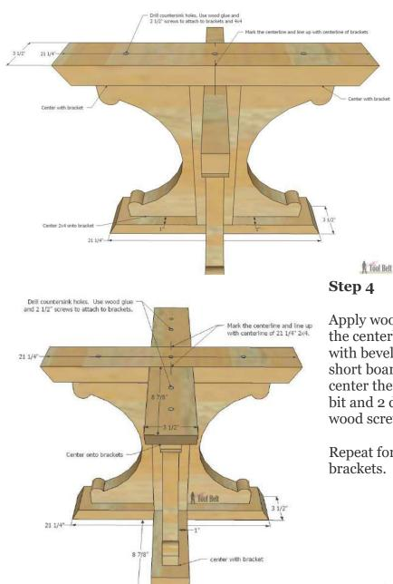
Apply wood glue along the top of the brackets. Mark the centerlines of the 2x4 -21 1/4" base long boards with beveled ends. Line up the centerline of the long board with the bracket centerlines, and center it along the brackets going the other direction. Use a countersink drill bit and drill holes, one in the center and one in each bracket. Use 2 1/2" wood screws to secure the base long board.
