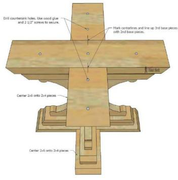
Repeat the process of steps 3 and 4. Apply wood glue along the top of the base layer 1. Mark the centerlines of the 2x4 - 21 1/4" base long boards and 2x4 - 8 7/8" base short boards with straight ends. Line up layer 2 long board on layer 1 short boards. Drill countersink holes in 3 places and secure with 2 1/2" wood screws.
