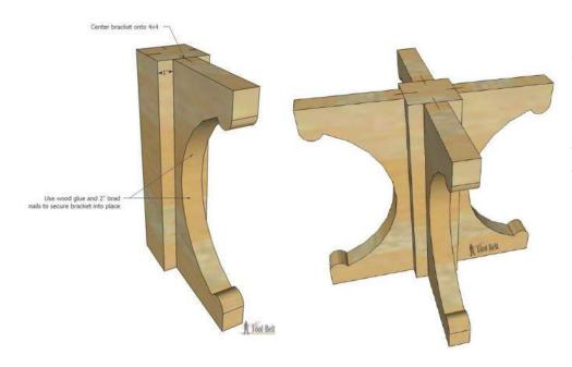
**Step 2** - Mark the centerlines of the 15 3/4" 4x4 ends and the bracket ends. Center bracket on the 4x4 and use wood glue and 2" brad nails to secure the bracket to post. Repeat for each bracket.
